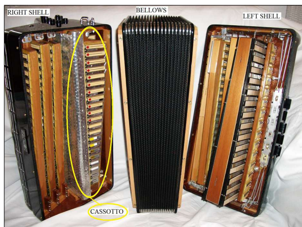
Figure 2. Layout of the blocks of reeds inside the accordion (front view). The cassotto or special resonance chamber that attenuates the higher harmonics (marked in an ellipse) is placed inside the right shell.
