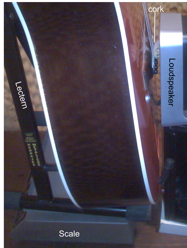
Figure 2. Experimental set-up. The three bass strings were struck using a sharp-edged cork glued to the cone of a loudspeaker in a soundproof room. The radiated sound was recorded using a couple of microphones, so that the 13 cm segment between them was located 100 cm in front of the top plate.
