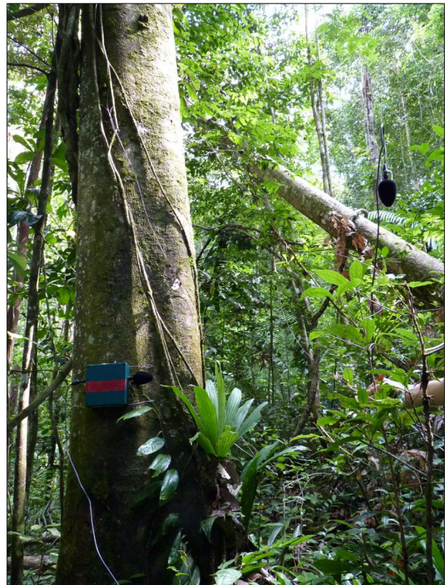
Figure 1. Field recording of acoustic communities or soundscapes. An autonomous digital recorder (SM2, Wildlife acoustics) is settled in the Nouragues tropical forest in French Guiana with one microphone at a human breast heights and one microphone ready to be placed in the canopy at a height of 20 meters. See [40] for details.
