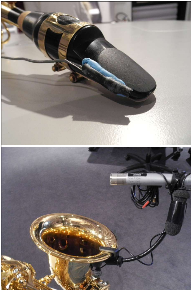
Figure 12. Top: Differential pressure transducer Endevco 8507-C1 used to measure the static pressure in the mouth. Bottom: Microphone B&K 2669 located at 15 cm from the bell used to measure the radiated pressure.
