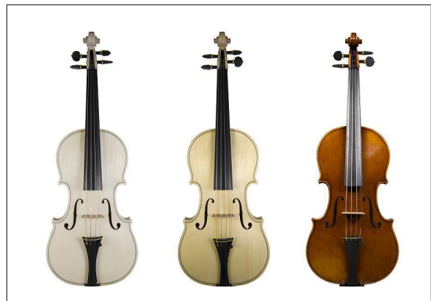
Figure 1. The violin in the three steps of the making process. Untreated (left), with ground coat (center) and varnished (right).
