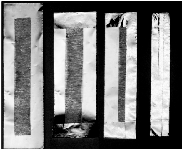
Figure 2. Folding of aluminum foil around optical lens cleaner film to create disbond.
