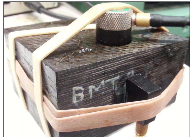
Figure 1. (Colour online) CFRP block in the test configuration with transmitting transducer on side and receiving on top.
