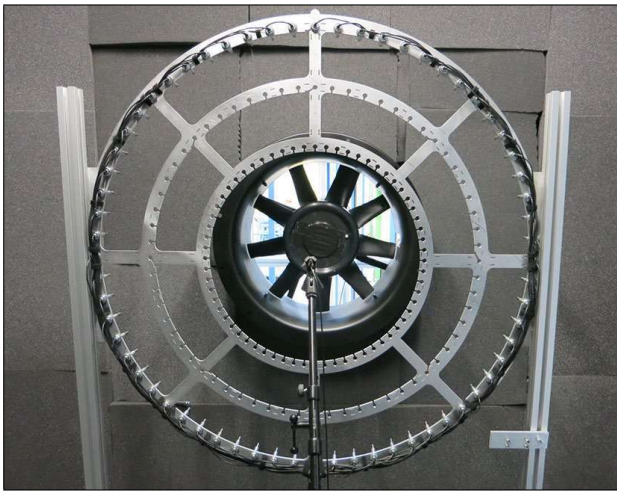
Figure 7. Generic test fan (rotational direction: clockwise) and microphone array.
