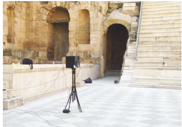
Figure 4. Typical source set-up for the acoustic measurements (source at position S_1 shown).
