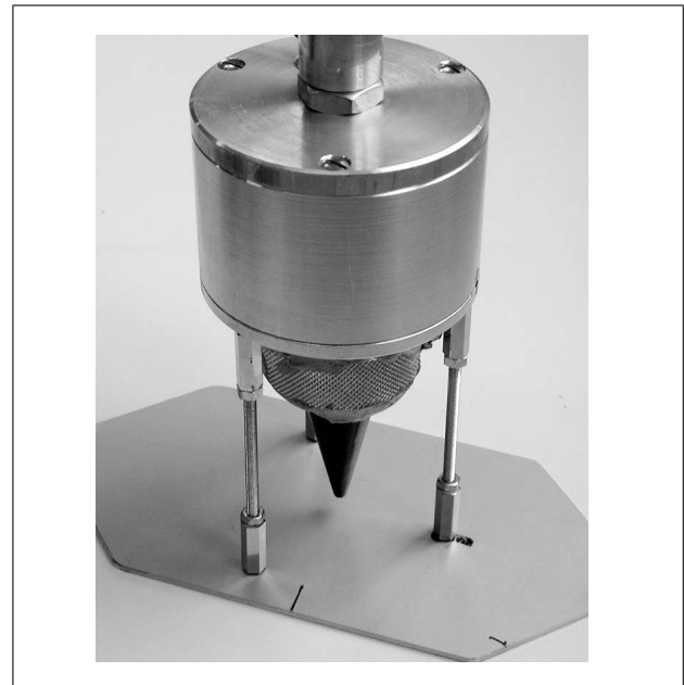
Figure 4. Source used for scale model experiments. The opening for sound radiation has a diameter of 2 mm and is located at the bottom end of the black cone.
