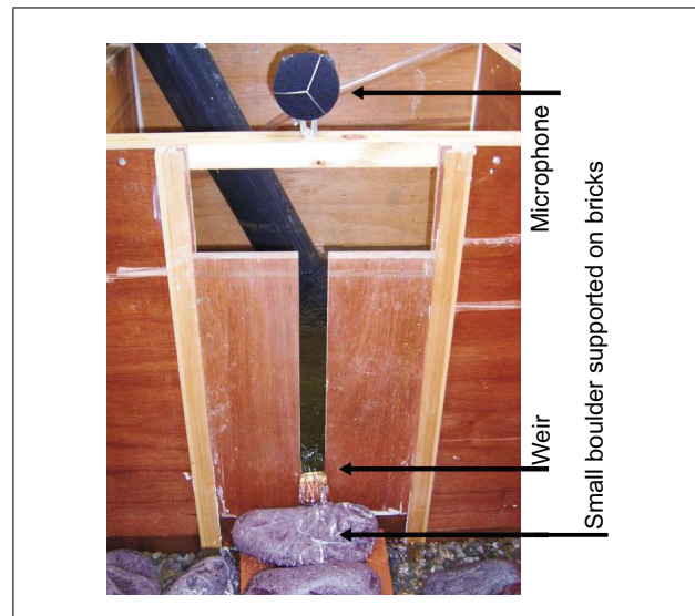
Figure 1. View of weir and microphone position in test apparatus.
