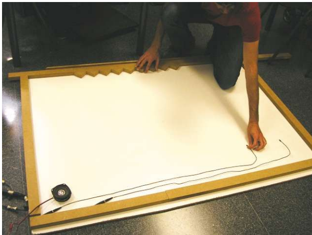
Figure 10. 1:5 scale reverberant chamber (2D) used for the measurement of the scattering coefficient of a set of nine triangles.
