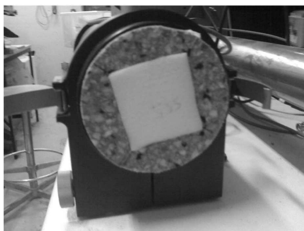
Figure 8. Example of an heterogeneous sample (u160 - melamine) in the Medium Kundt Tube.
