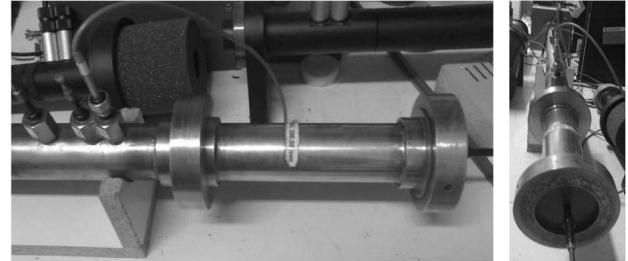
Figure 4. Small Kundt Tube. Left: front view, right: top view.
