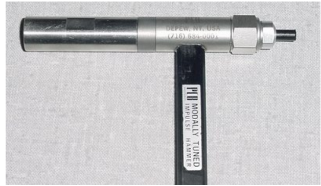
Figure 17. Example of a hammer with cylindrical tip of PE, adapter for the tip, force cell, intrinsic mass and additional mass.
