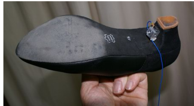
Figure 13. Reference shoe with mounted accelerometer.
