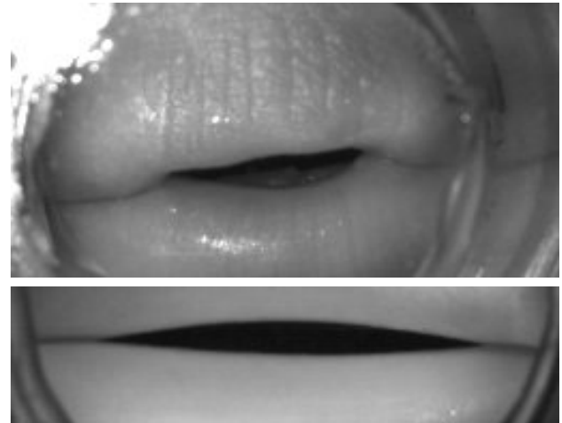
Figure 7. Maximum width of the opening of the lips of (top) player TJ playing the note Bb 2 at mf and (bottom) the artificial mouth playing note E 3 at 97 dB.
