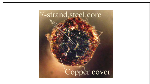
Figure 3. Shanghai second string microphotograph cross-section with plastic cover removed.
