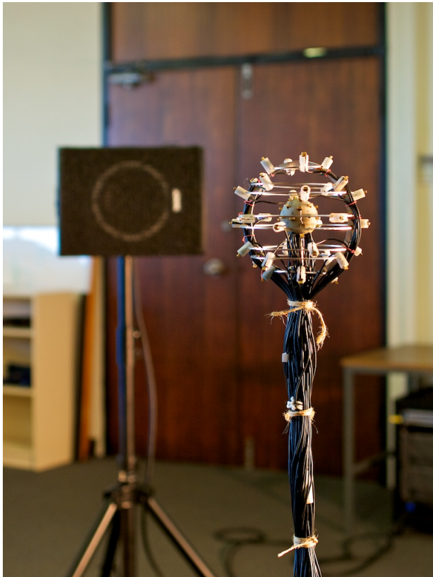
Figure 10. A photo is shown of the dual-radius spherical microphone array being measured in an office at the University of Sydney.
