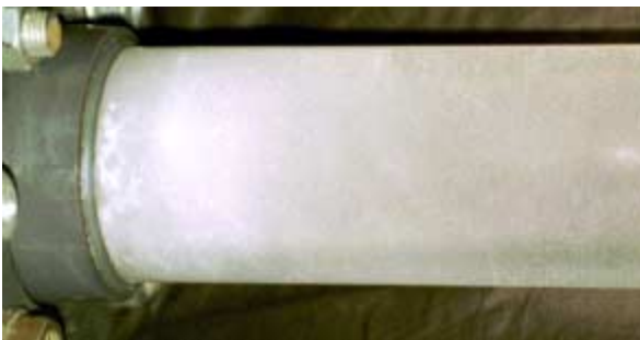
Figure 6: Example of chocking cavitation with a large pocket of micro bubbles downstream of the valve.
