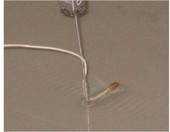
Figure 4. Optical observation for the calibration of the zero level in the measurement of the depth.
