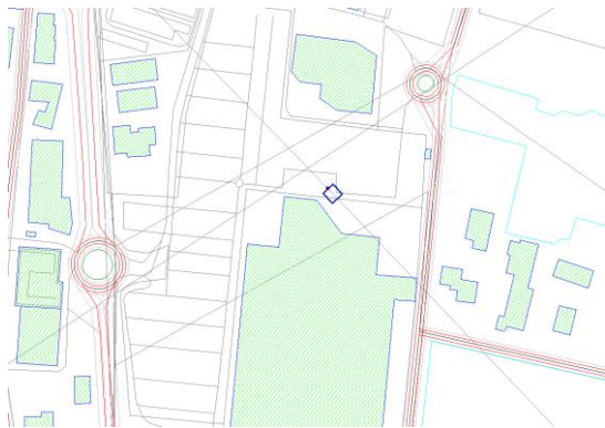
Figure 2: Map of the neighbourhood considered for the acoustic modelling. The blue square in the middle is the CSP shelter.
