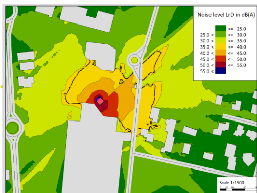
Figure 10: Noise map of the area surrounding the shelter at 2 m above the ground.
