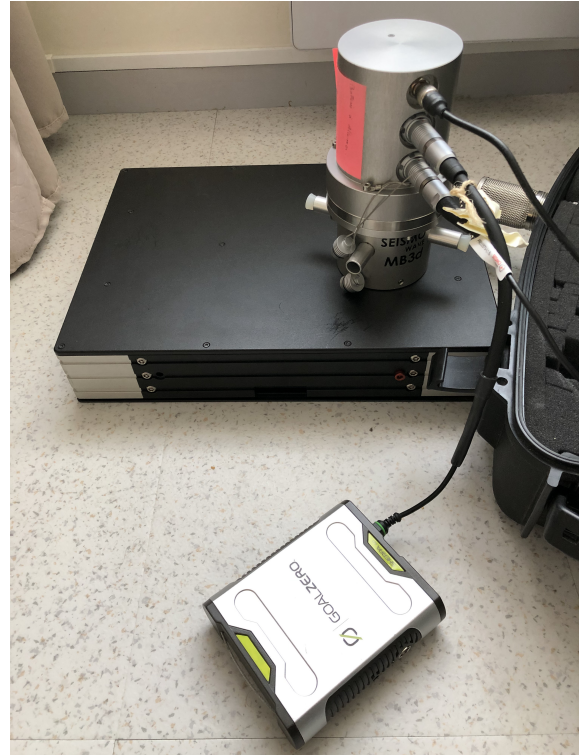
Figure 1. Recording setup. The digital MB3d sensor, placed on the anti-vibration device, is powered by an external battery.
