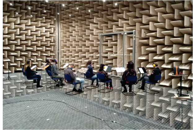
Figure 3. Measurement in anechoic chamber, loudspeaker and microphone pairs on the sides of the picture.
