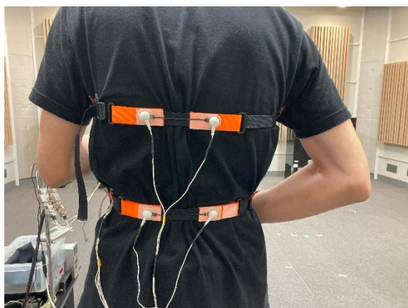
Figure 2. belts with elongation sensors to measure the abdominal motion and chest motion.
