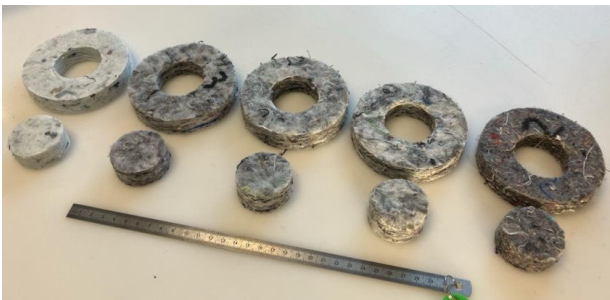
Figure 1. Impedance tube samples (Ø45 mm) extracted from AFR samples (Ø100 mm) for different mixtures.
