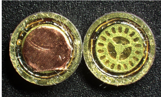
Figure 6. A circular piece of copper tape is attached to the speaker membrane. Increasing the moving mass by 2.5 mg
