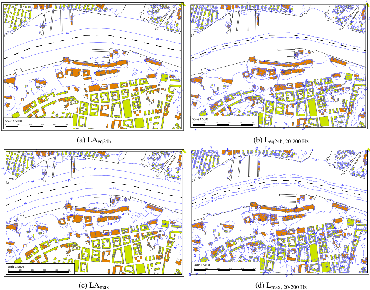
Figure 7: Calculated noise contours along a section of the river where to ro-ro ferries pass four times a day. Contours are presented for both a-weighted levels (left) and for low frequency levels (right). Residential buildings are green and other buildings are orange.
