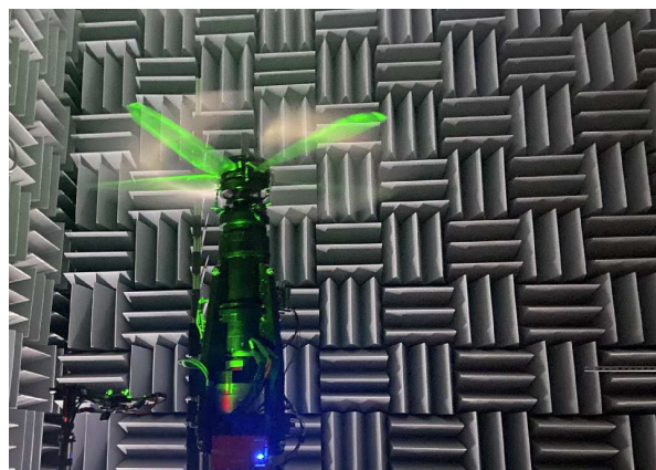
Figure 2. Testing of the notional UAM rotor with five blades.
