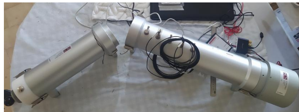
Figure 2. Impedance tube used for measuring the absorption coefficient.
