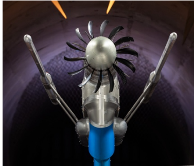
Figure 1. Picture of the open fan model with two arms of microphones and in S1MA wind tunnel
