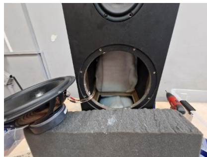
Figure 2. Test enclosure – polyester fibers variant
