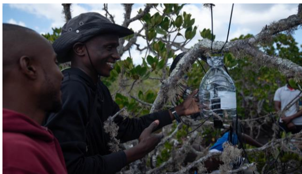
Figure 6. Microphone hung on a higher branch in order to record air sounds, covered to avoid disturbance from wind and rain (Photo by Enrico Nicosia).
