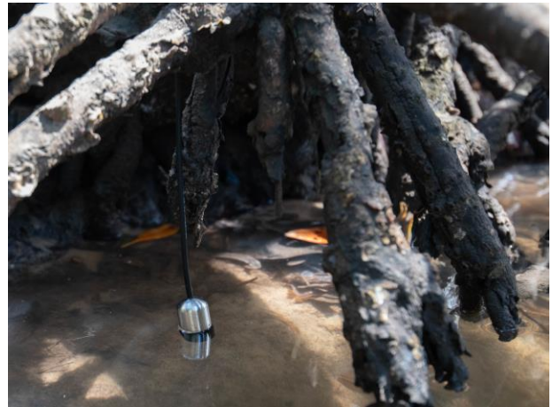
Figure 4. Hydrophone hung on the roots in order to be outside of the water with the low tide and submerged with the high tide (Photo by Enrico Nicosia).
