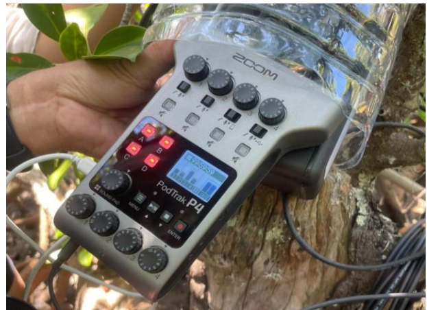
Figure 5. Recorder: as inputs, we used one microphone for air and three hydrophones for water and soil (Photo by Aura Rapino).
