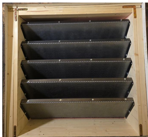
Figure 4. Tested louvered noise barrier from room for outgoing sound.
