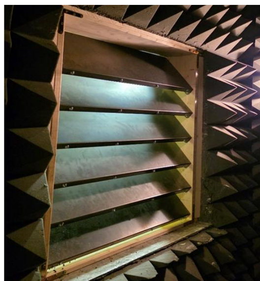
Figure 5. Tested louvered noise barrier from sound receiving room.
