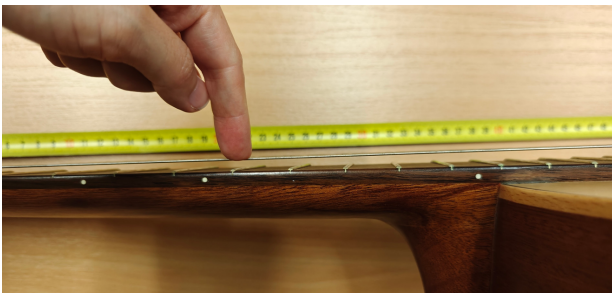
Figure 1. Classical guitar with side dots placed slightly left from the positions of 1/2 , 1/3 and 1/4 on the string (from right to left). The finger is placed lightly touching the string on the fret that corresponds to 1/3 of the string.
