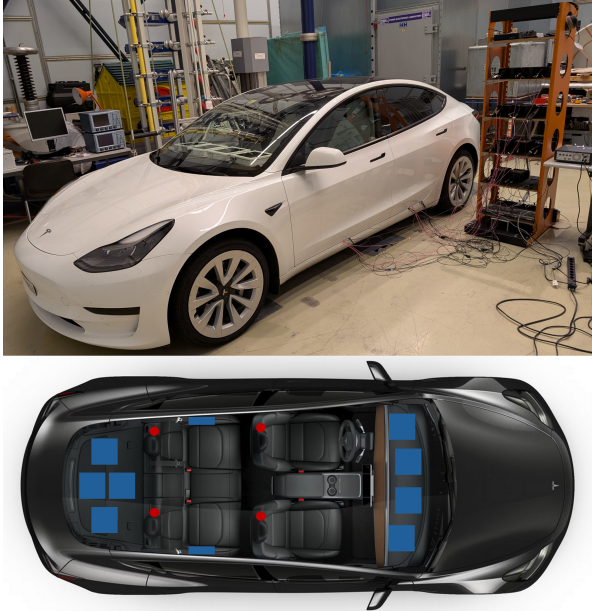
Figure 2. Vehicle under test with 10 plasmacoustic transducers placed in the cabin above; schematic locations of the microphones (red dots) and plasmacoustic transducers (blue rectangles) below.
