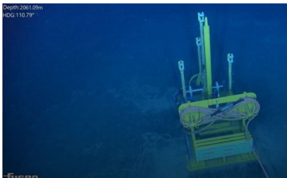
Figure 3. Screenshots of the FRUGRO ROV during the installation of the IPANEMA-CT acoustic observatory. The image shows the four hydrophones of the frame arranged in a tetrahedral configuration, with a depth exceeding 2060 m.
