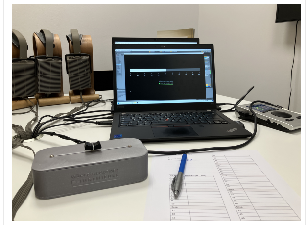
Figure 3. Experimental setup with mechanical slider, visual feedback and questionnaire
