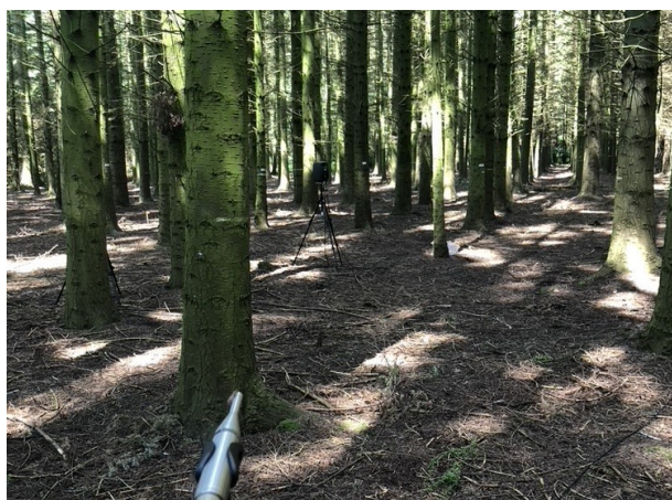
Figure 2. The forest environment considered in this study. The measurement setup can be seen: an Earthworks M30 omnidirectional measurement microphone and a Genelec 8130A loudspeaker.
