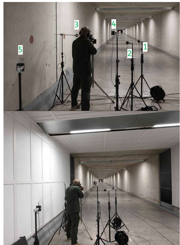
Figure 2. Measurement set-up using 5 microphones close to hard walls (upper) and absorbing walls & ceiling (lower).
