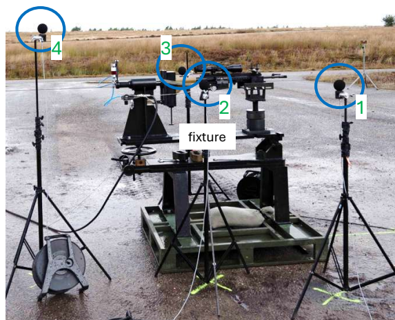
Figure 4. Outdoor measurement using a weapon fixture.
