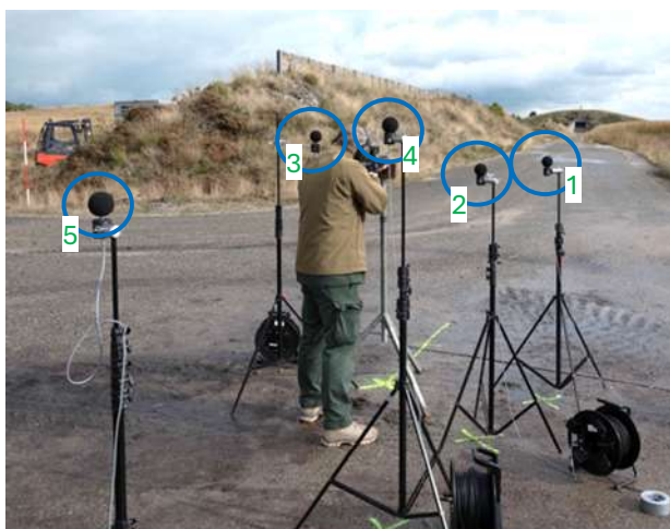
Figure 3. Outdoor measurement set-up using 5 microphones.
