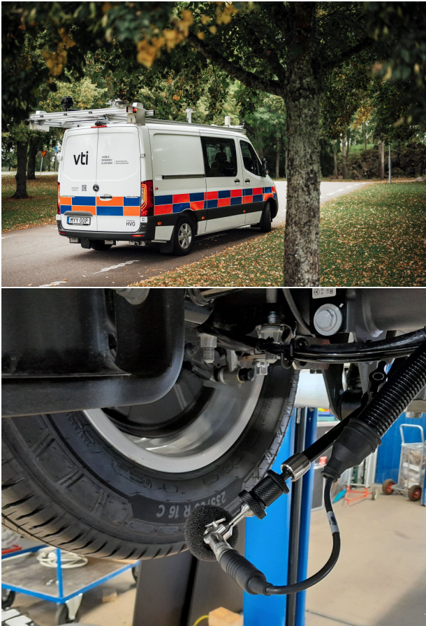
Figure 4. The VTI Mobile Research Platform (top, ©Satu/VTI) with the microphone for exterior sound recording mounted close to the left rear wheel (bottom, ©Ramboll).
