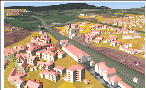
Figure 3. Automatically generated facade points from LoD2 building data and spatially evaluation of noise immission (©DB InfraGO AG).
