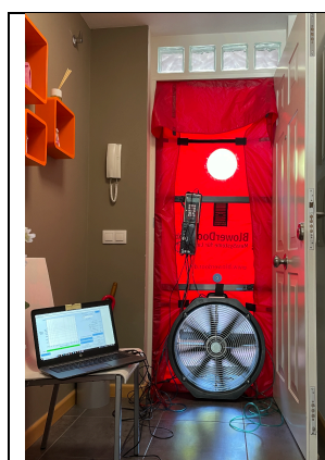
Figure 4. Blower Door setup – House 1
