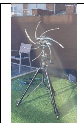
Figure 5. Microphone arrays and the camera setup
