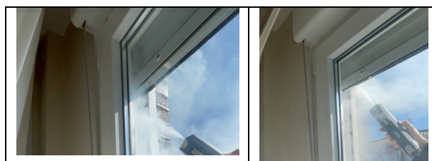
Figure 8. Visual identification of air leakage locations in House 1 using smoke generator
