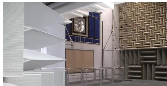
Figure 3. Inlet plenum of the anechoic test facility with fan mounted in separation wall.
