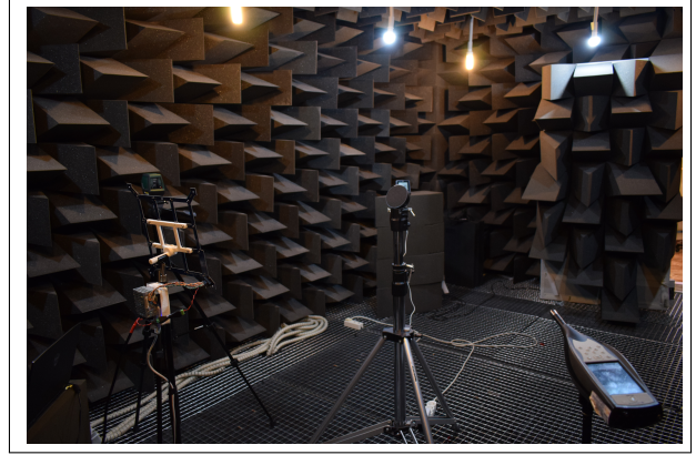
Figure 4. SGA positioned at one meter from the sound source. A sound frequency analyzer was placed at a fixed position to control the sound source's stability.
