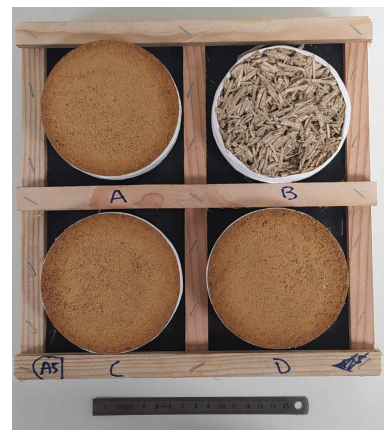
Figure 1: Formulation example with three coated samples (A, C, D) and one uncoated sample (B).
