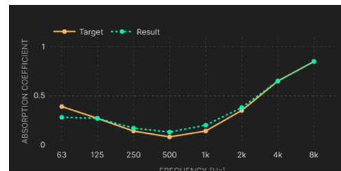
Figure 5: Estimation of the absorption properties of the material after a fitting process inside Treble software.
