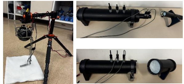
Figure 3. Measurement systems used in the present investigation: in-situ PU method (Left), and impedance tube (right).
