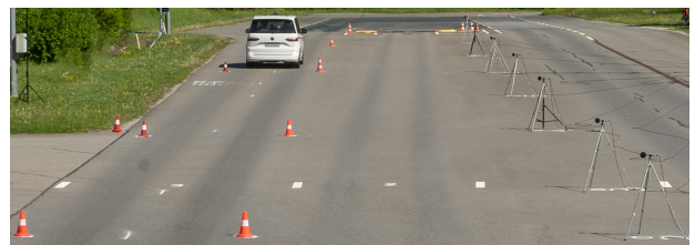
Figure 1. Photo of the test track and measurement setup. Seven microphones (right) are capturing exterior noise from the VW Multivan T7 passing by.
