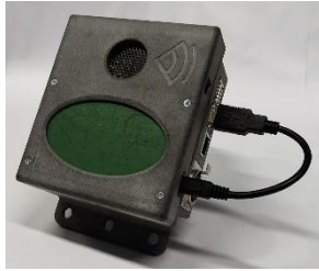
b) The CoSys-Lab eRTIS sensor [8] in a custom enclosure.
