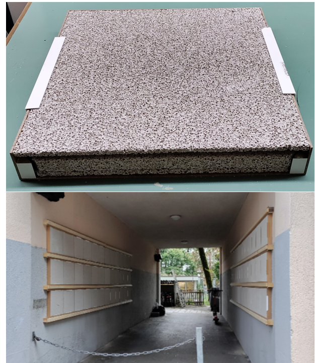
Figure 1. Top: layered setup of the optimized absorber panel. Bottom: Placement of the absorber panels in the courtyard entrance.
