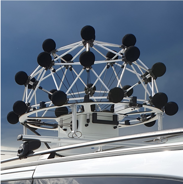
Figure 7: JR-IcoDome32 with GNSS-IMU module mounted onto the rack roof of a car for mobile use.
